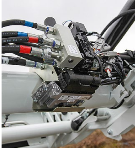
The control equipment mounts on the loader crossbar (the guard is removed for the pic).
