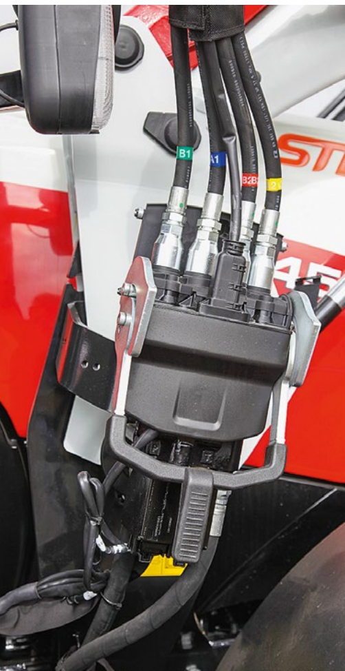
The multi-coupler works under pressure and has a rotatable fitting on the loader side.
