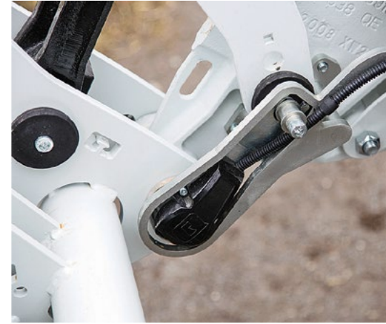
Angle sensors measure the position of the loader boom and the attachment. The data can then be stored and retrieved automatically.
